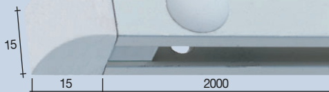
Schiene, Alu weiß pulverbeschichtet | 2 Rail, white, powder coated Rail poudre époxy blanc
